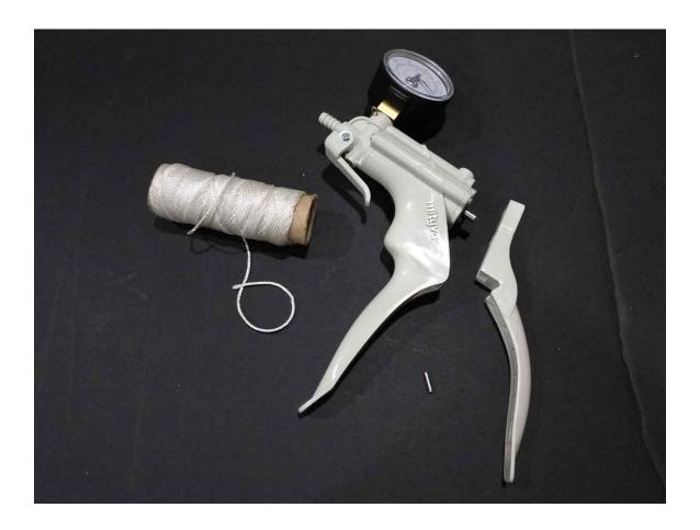
**1. Things you'll need:** The parts of your hand pump, and a piece of string. A nylon construction string works nicely,
