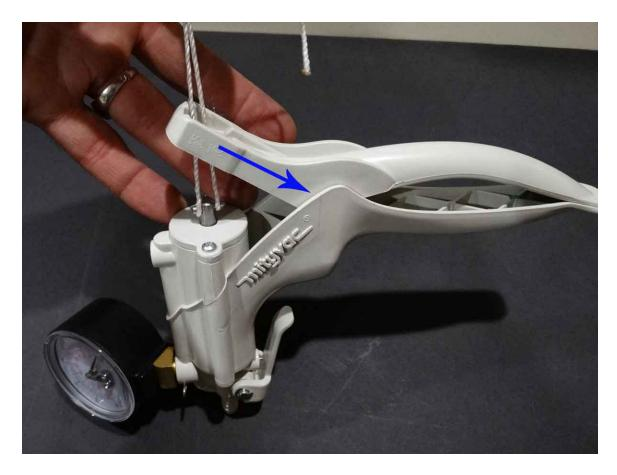
6. Seat the moving handle in place at it's pivot notch.
