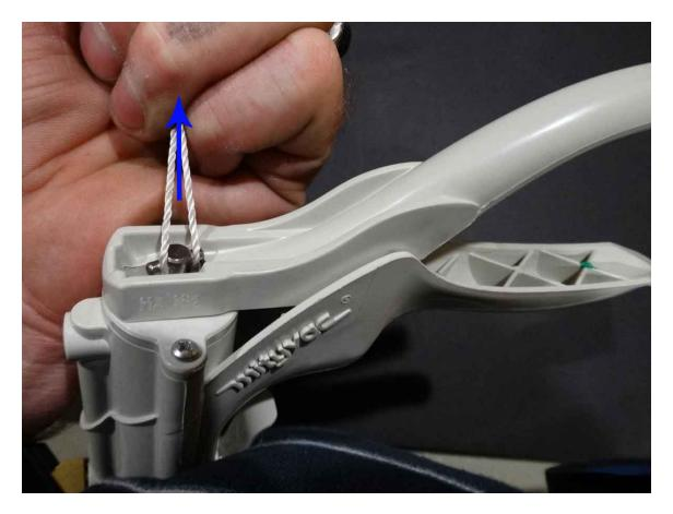
7. Tilt the top edge of the moving handle down over the pin and shaft, then pull straight upwards so the pin and shaft end extend past the handle a little ways.
