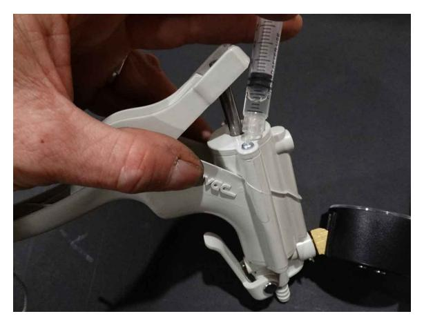
13. A few drops placed on the back of the shaft also wouldn't hurt. Operate the handle again several times to help distribute the oil inside the pump. Wipe off any excess oil that remains, and you are done.
